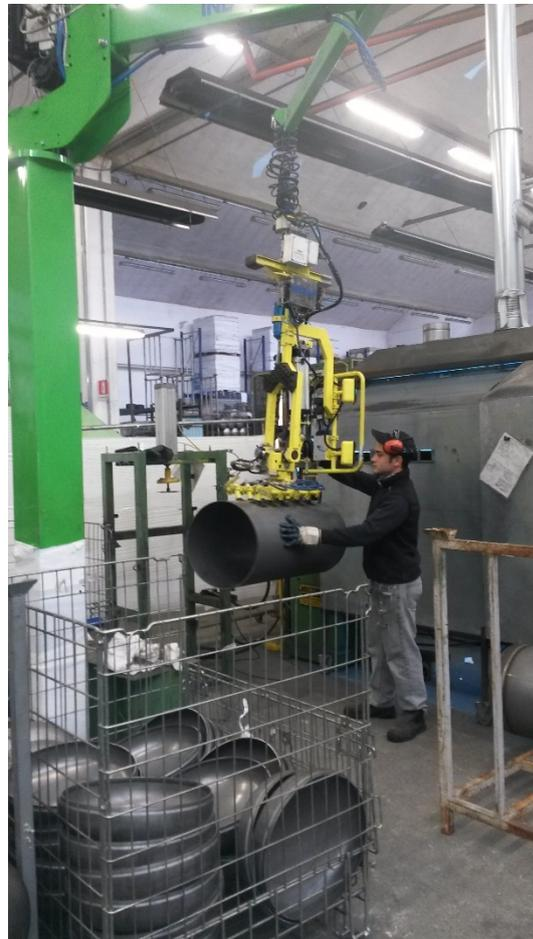
Picture2: Indeva Liftronic® with custom gripper
