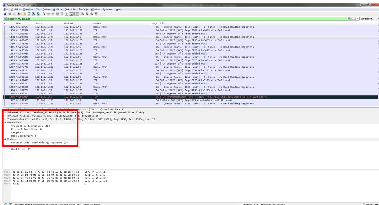
Picture 3 - Analysis of network traffic and identification of the communication protocol used
