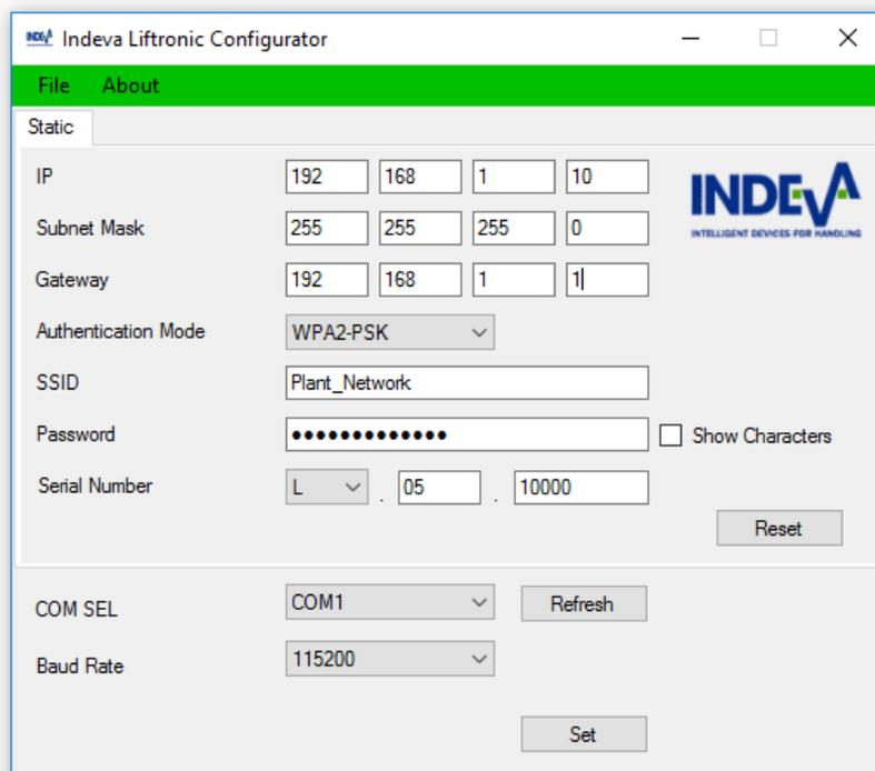
Picture 5 - IP address configuration and network parameters
