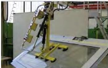
Vacuum tool for lifting doors with 90 degree inclination
