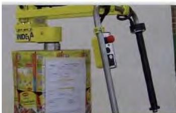
Electronically activated reel gripper
