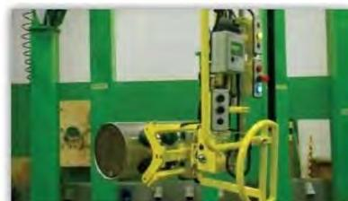
Vacuum gripper for lifting vehicle exhaust assembly with 90 x 90 degree rotation
