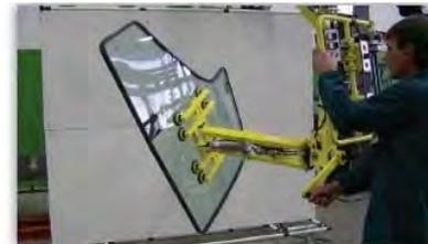
Vacuum tool for lifting vehicle glass with 180 degree manual rotation and auto centre of gravity
