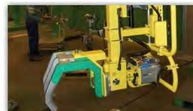
Pneumatic gripper for picking cylinders with 180 x 180 degree manual rotation
