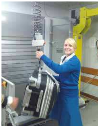
Air and electric connections via a continuous swivel joint at the toolhead to keep cables from tangling.
